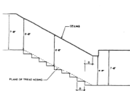
Figure 1009.2 STAIRWAY HEADROOM REQUIREMENTS
