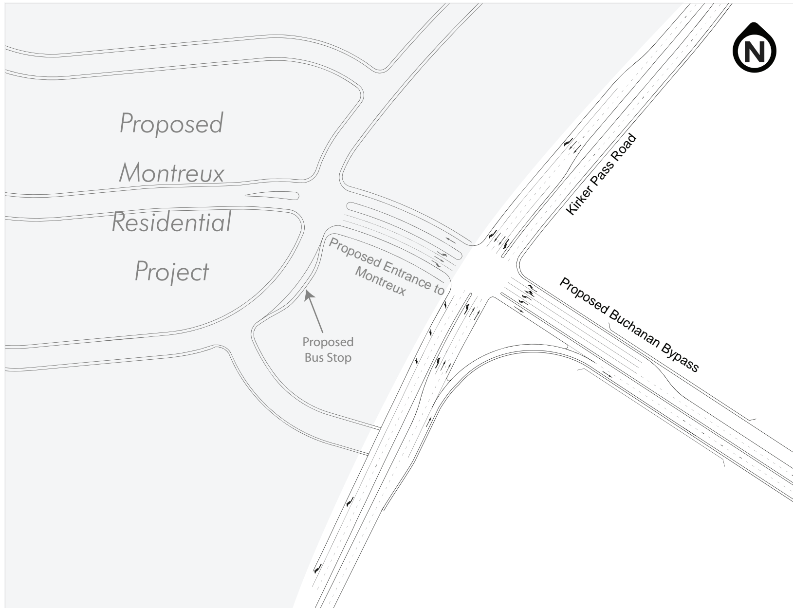
FIGURE 11 | PRELIMINARY DESIGN FOR THE BUCHANAN BYPASS CONNECTION TRAFFIC IMPACT STUDY Montreux Residential Project City of Pittsburgh
