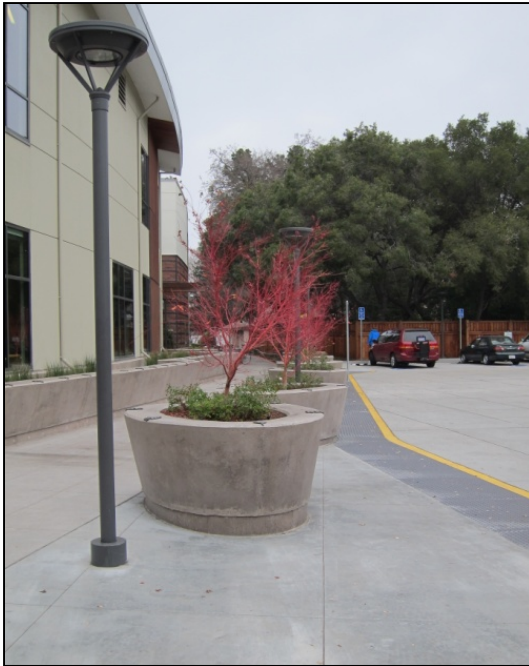
Pick-up/Drop-off Area at the Same Elevation as Sidewalk in Walnut Creek, CA
