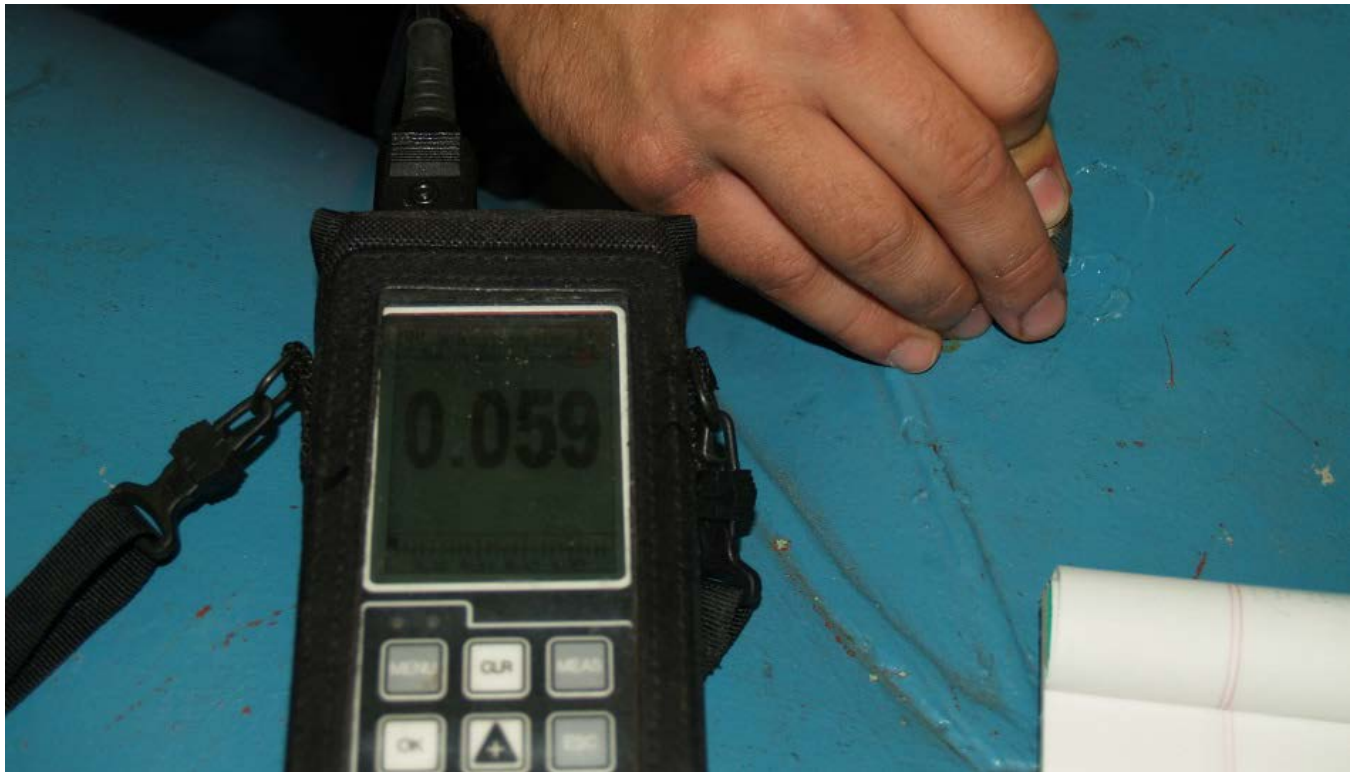
Figure 2-7. Filter 8 Outlet Tee with Ultrasonic Thickness Gage
