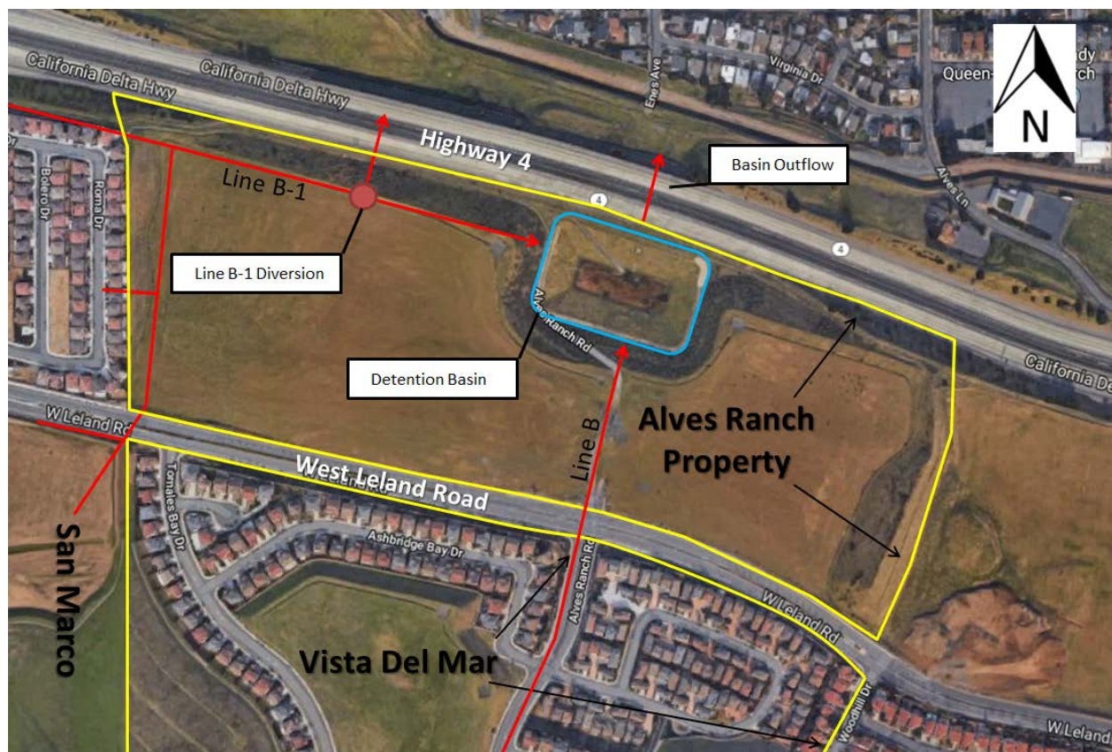
Figure 1: Schematic and Aerial Map of Basin, Storm Drain Lines, and Flow Directions.
